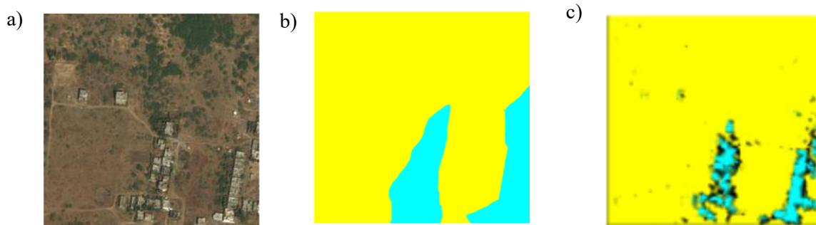
РисFig. 7. Example of satellite image segmentation: a) original image; b) marked mask; c) segmentation result
