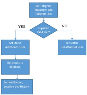
Figure 1: Algorithm of telegram bot
