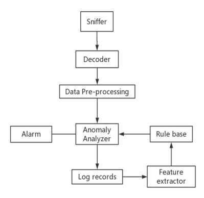
Figure 1: Model of intrusion detection based on data mining
